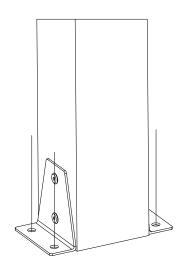
**8)** Once the Arch is in the Desired Location, Support or Add Braces to Hold it Upright While it is Anchored to the Ground. Using Anchors (not included) Appropriate for the Anchoring Surface, Secure the Arch Using (2) Anchors in Each Metal Angle Bracket
