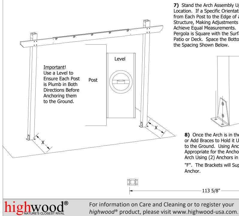
7) Stand the Arch Assembly Up and Move to the Desired Location. If a Specific Orientation is Desired, Measure from Each Post to the Edge of an Adjacent Surface or Structure, Making Adjustments to Each Post as Needed to Achieve Equal Measurements. This Will Ensure the Pergola is Square with the Surface it Sits on, such as a Patio or Deck. Space the Bottoms of the Posts to Ensure the Spacing Shown Below.
