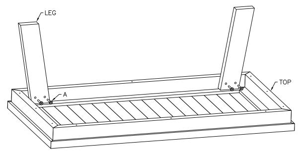
Attach the Legs to the Top using two A bolts in each leg
