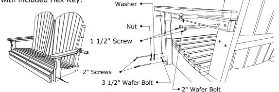
3. Attach short end of chain to Back & long end through screw eye to bottom of front upright. Always use
