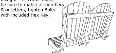
2. Attach (C) Armrest's using 1 - 2" Wafer Bolt 1 - 3 1/2" Wafer Bolt 1 - Washer 1 - Nut 2 - 2" Screws & 2 - 1 1/2" Screws per side, be sure to match all numbers & or letters, tighten Wafer Bolt with included Hex Key.
