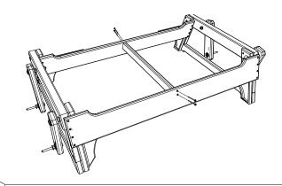
3. Attach (D) Bearing Arm Supports to Glider Base using 4 - 2 1/2" Screws per side, be sure to match all numbers & or letters.
