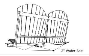
7. Attach Back-Seat Assembly to Armrests using
