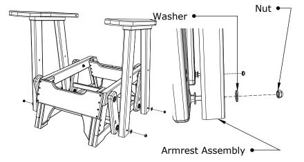
5. Attach (B) Back Assembly to (A) Seat Assembly using 1 - 2" Wafer Bolt in top hole per side, Be sure to match all numbers & or letters. Tighten Wafer Bolts with included Hex Key.
