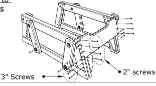
2. Attach (I) Cross Pc. to Inside of Glider Base ◆ 2" Screws Sides using 4 - 2" Screws and 3 - 3" Screws per side, Be sure to match all numbers & letters. 3" Screws
