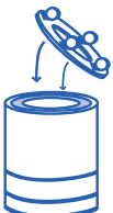
Position the indentation in the cover into the center of the HEPA filter
