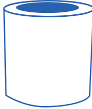
26 lbs impregnated Carbon filter 17% potassium iodide carbon, 83% coconut shell 24 months
