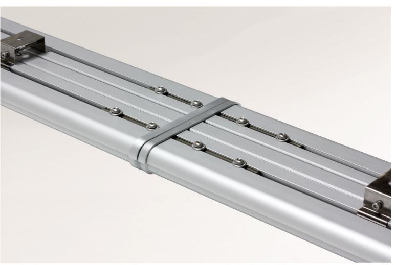
The Rezista Planus has a pendant way of installation. The metal clamps can be positioned at any position, giving the installer freedom of installation. The metal clamps are extra secured by a horizontal shoulder bolt. The seamless connection of the 2 fixtures is done by 2 metal plates and secured by 8 screws.
