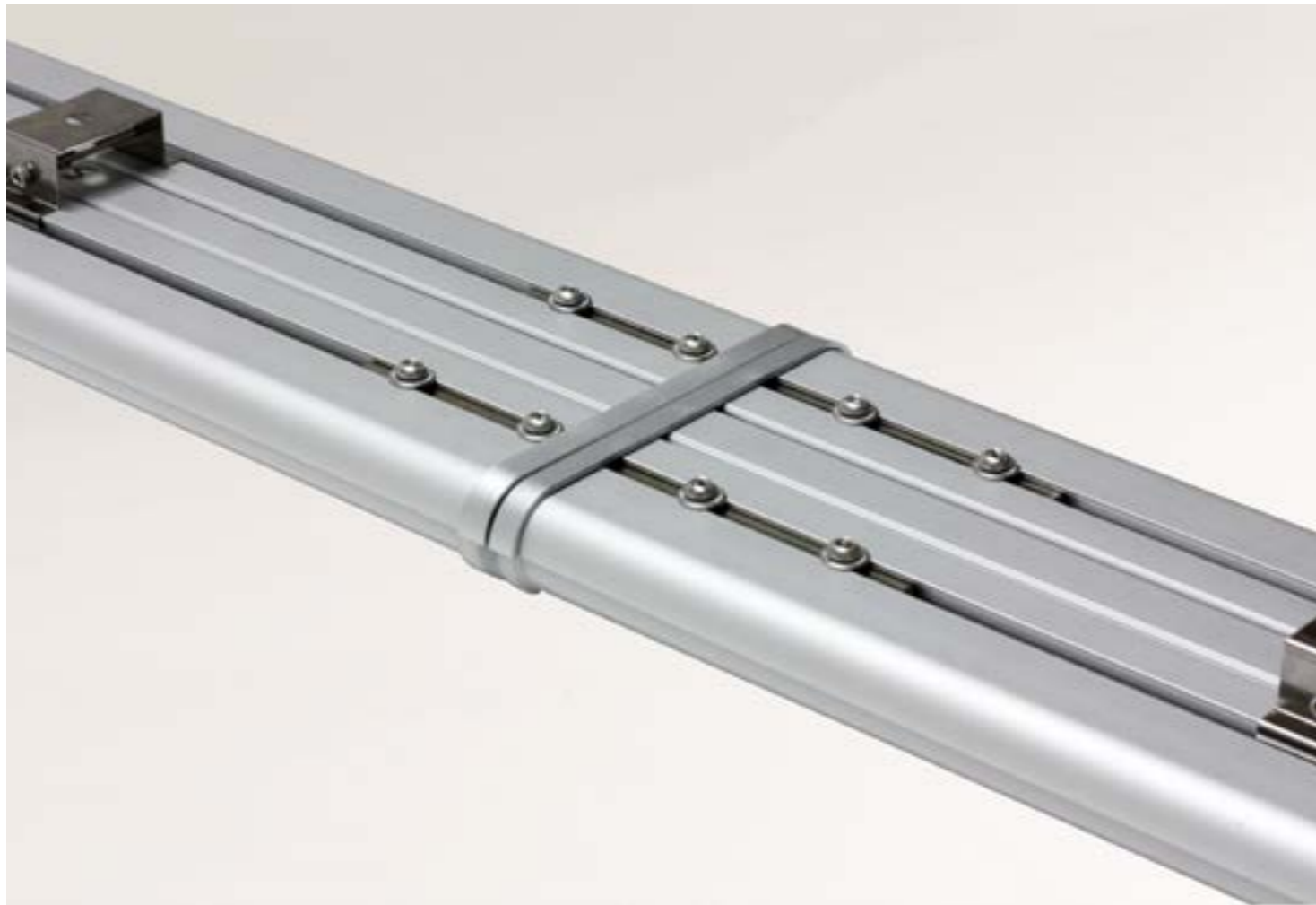
The Rezista Planus has a pendant way of installation. The metal clamps can be positioned at any position, giving the installer freedom of installation. The metal clamps are extra secured by a horizontal shoulder bolt. The seamless connection of the 2 fixtures is done by 2 metal plates and secured by 8 screws.
