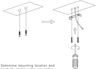
Determine mounting location and knock the plastic anchor into ceiling, fix bracket with screw into the ceiling.
