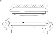
Match the gaps for each part and rotate the frame clockwise.
