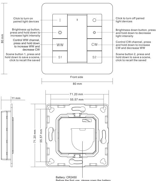
Before the first use, please open the battery cover and remove the protective film
