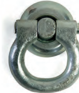
RECESSED LASHING RING 2 • Universal joint for loading in any direction • Weld around entire circumference when fitting • Forged steel ring • Can be supplied with seal plates, rubber seal and pan if required • 2000 daN (kg) permissible tensile load • Zinc plated finish
