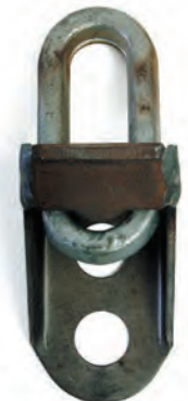
RECESSED LASHING RING 3 • Designed to be recessed at floor level • Designed for ease of assembly to trailer frame by webbing, forming integral part of structure • Main body self colour, ring galvanised • 3000 daN (kg) permissible tensile load
