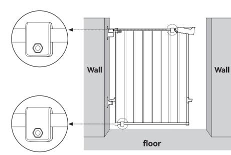
Extend the door rail to the wall and determine the sticking position of D and E
