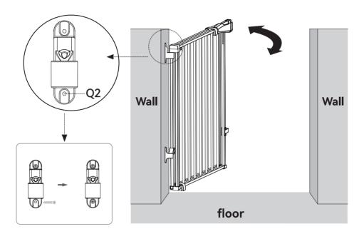
Adjust the width of the door frame again, so that the distance between the handle and the upper latch is less than 0.078in, and then lock the E- latch
