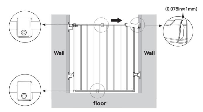
2 Open the door frame, install the upper latch and lower latches
