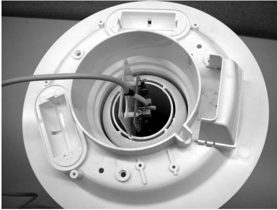
Installing the Temp/Hum Sensor
