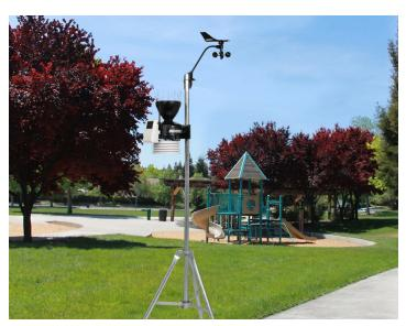
Vantage Pro2 on Mounting Tripod
