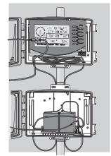
Cabled Vantage Pro2 ™console mounted in Extra Solar Power Kit (top) with Heavy Duty Solar Power Kit (6612, bottom)
