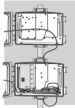
Wireless Weather Envoy™ mounted in Solar Power Kit (6614, bottom) with Extra Solar Panel Kit (top)
