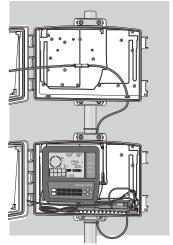
Vantage Vue Console mounted in Solar Power Kit (bottom) and Extra Solar Panel Kit (top)
