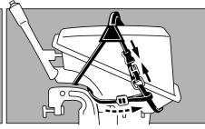
Slide the security strap's large loop onto the main harness. Close harness attachment buckle (as in third step, above). Tighten harness and security strap webbing.
