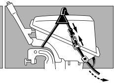
The harness may be installed with buckle on either side of motor. The webbing is one continuous piece; pulling on one side will tension the other side.
