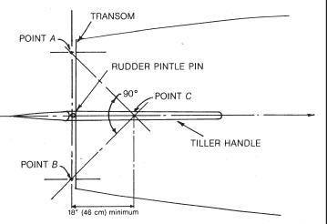
Assemble the Tiller-Tamer unit to the tiller handle by positioning the knob over point C. Attach with two wood screws provided. Release the knob and thread the 1/4" (6.4 mm) line through as shown below.
