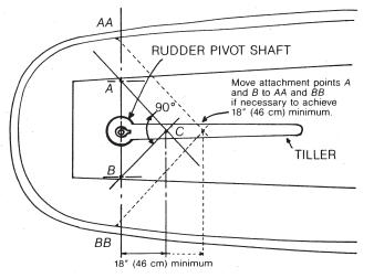
Assemble the Tiller-Tamer unit to the tiller handle by positioning the knob over point C. Attach with two wood screws provided. Release the knob and thread the 1/4" (6.4 mm) line through as shown below.
