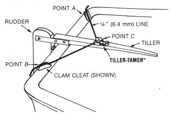
**4.** Attach a cleat at points A and B. This may be a clam cleat or any other quick releasing device. CL201 is recommended, as shown in previous drawing..
