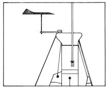
Mounting a wind indicator clear of VHF antennas, lights, or other installations.
