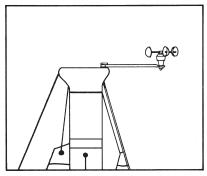
Mounting other accessories such as wind velocity sensors away from mast turbulence.
