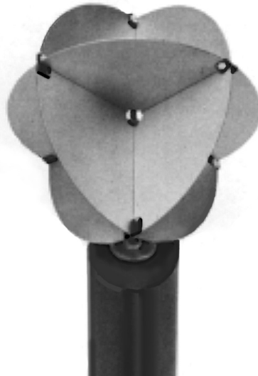
Rigid mounting on a mast structure using pipe fittings. Simple instructions for such a surface mount system are given later in this document.
