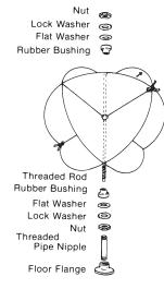
**Figure 3.** Permanent or hard mounting.
