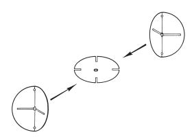
**4.** Important: After assembling radar reflector, securely lash two corners using 1/16" (1.6 mm) synthetic line.
