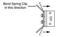
Remember to install the split ring in the hole on the shaft after it has been positioned in the spring clip.
