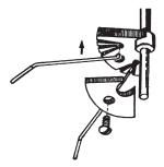
2. Slide vane onto shaft, add nylon washer. Captivate with collar. Secure collar on shaft with #4 set screw.
