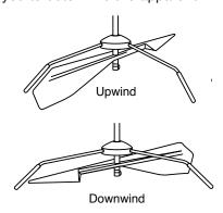
Three different detent positions are provided: 60°, 90°, and 120°. The 90° position is a good angle to use for general purpose sailing. The following guidelines may allow you to set the angle more precisely:
