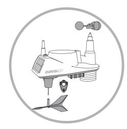
Assemble the Vantage Vue Integrated Sensor Suite (ISS) by attaching wind cups, wind vane and rain measuring mechanism. (Pages 1-4, Weather Box User Guide)
