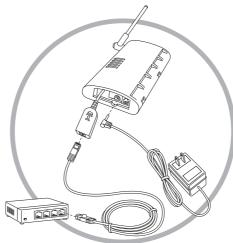
Connect Weather Envoy to router and AC-power adapter. (Pages 5-8, Weather Box User Guide)
