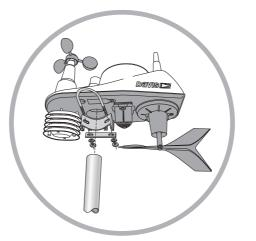
Mount the ISS to a freestanding or rooftop pole using the included U-bolt clamp (pole not included). (Pages 12-16, Weather Box User Guide)
