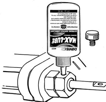
4. After lubricating, reconnect steering linkage.
