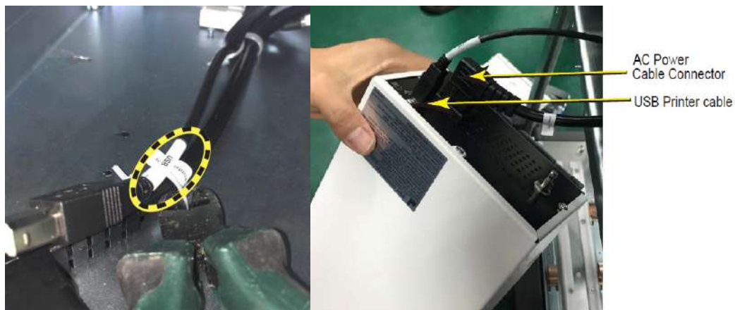
Figure 3-11. Connect printer power cable and USB cable
