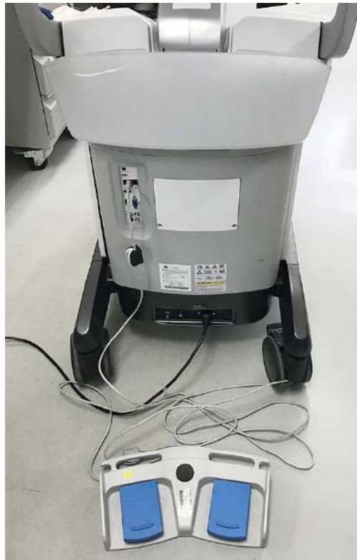
Figure 3-29. Connect Footswitch to the system (1)
