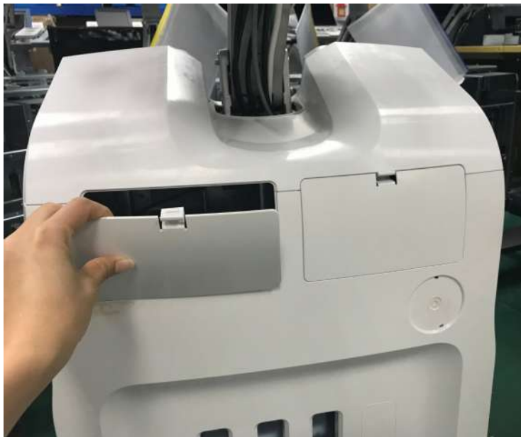
Figure 3-36. Remove printer and ECG cover
