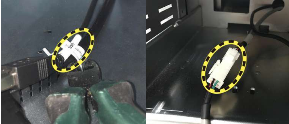
Figure 3-24. Connect DC printer power extension cable
