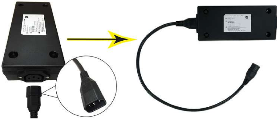
Figure 3-51. Insert the cable into the EMI filter output side
