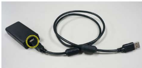
Figure 3-48. Insert the USB connector into Printer USB Isolator
