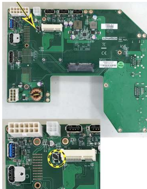
Figure 8-12. Debug Button on IODKG
