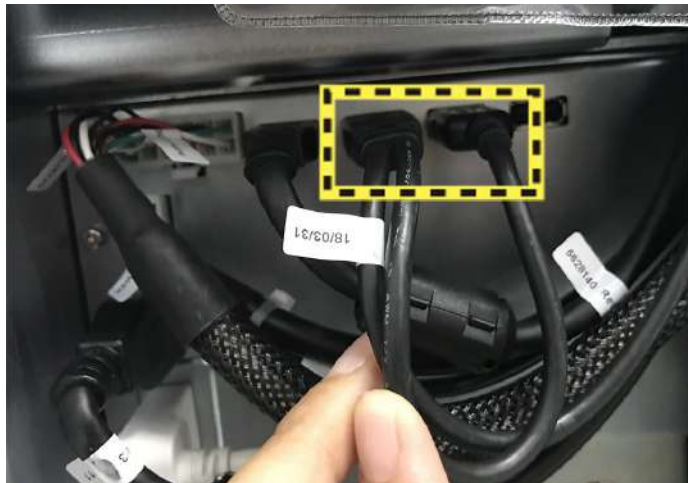
Figure 3-40. Connect both of the DVD USB cables
