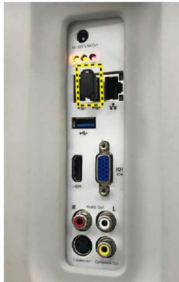
Figure 3-42. Connect Bluetooth Adapter
