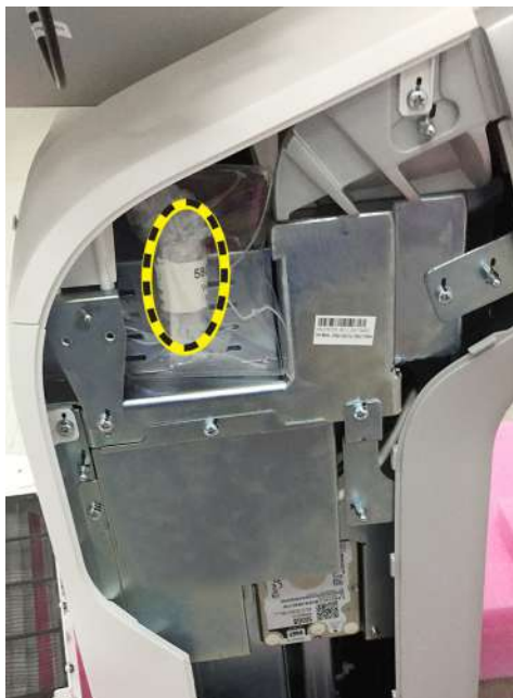
Figure 8-26. Software USB memory stick position
