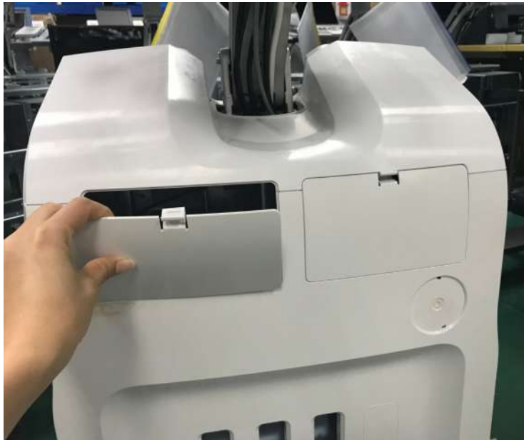
Figure 3-22. Remove printer and ECG cover
