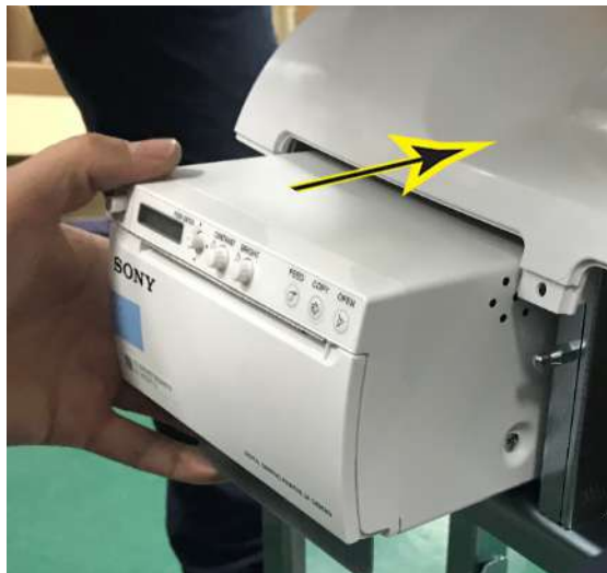
Figure 3-26. Insert DC printer
