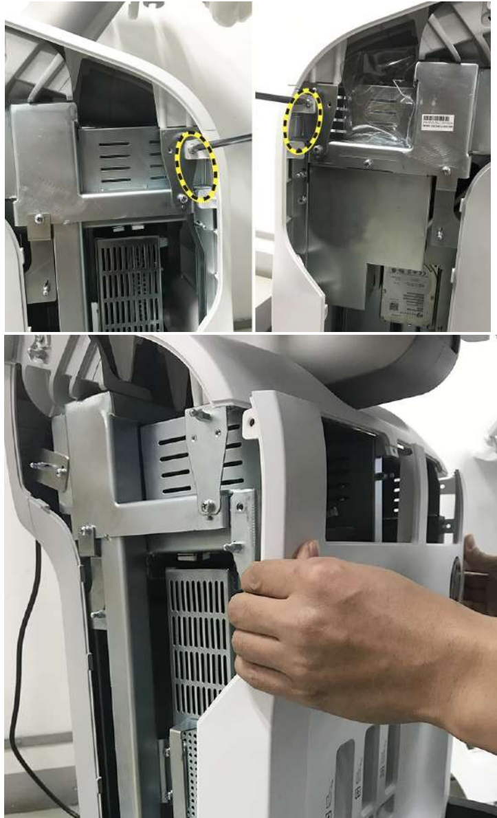
Figure 3-23. Remove body 4PP/3PP cover Assy
