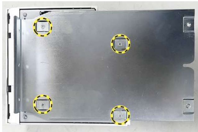
Figure 3-20. Install printer to printer shelf
