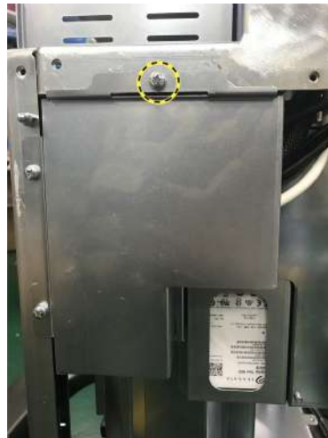
Figure 3-39. Remove the metal sheet
