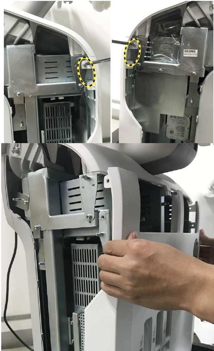
Figure 3-37. Remove body 4PP/3PP cover Assy
