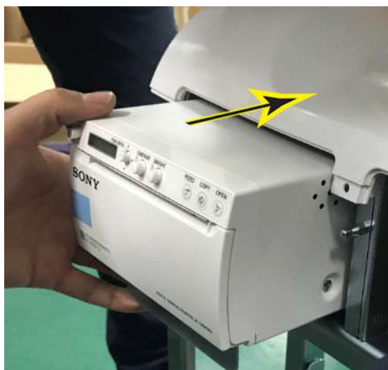
Figure 3-12. Insert AC printer
