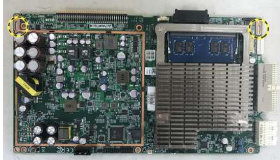
Figure 8-10. Install CWI PWA with CMOS battery
