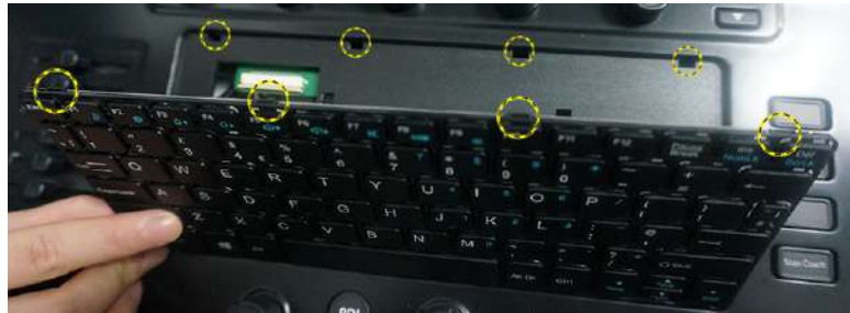
Figure 8-4. Install AN Keyboard
