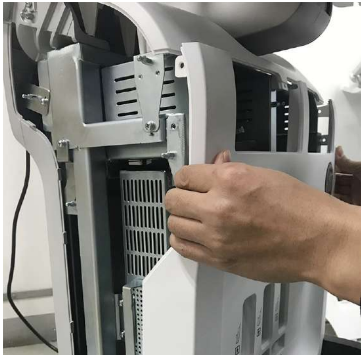
Figure 3-10. Remove body 4PP/3PP cover assy
