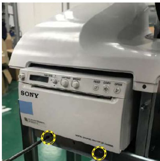
Figure 3-27. Push the printer assembly
