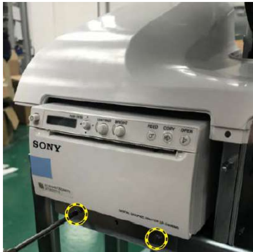
Figure 3-13. Push the printer assembly
