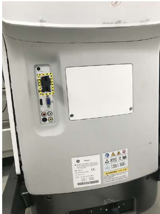
Figure 3-41. Connect Wireless Adapter
