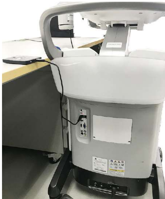
Figure 3-32. Connect HDD to the system
