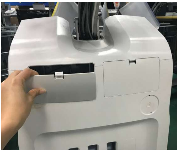
Figure 3-9. Remove printer and ECG cover
