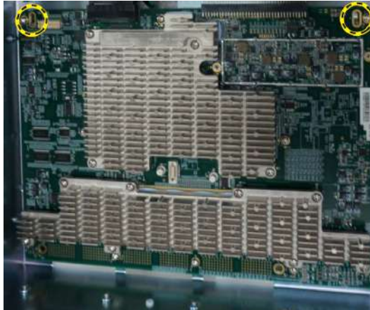
Figure 8-8. Install MST PWA Assy (1)
