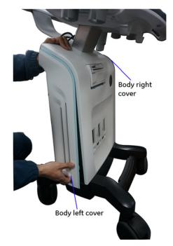
Figure 3-24. Remove the body left cover
