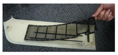
Figure 3-25. Remove the Filters
