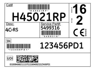
Figure 4-5. Probe box label
