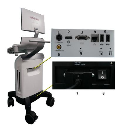
Figure 1-2. Peripheral/Accessory Connector Panel
