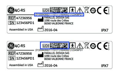
Figure 4-6. Probe Label UDI GTIN and Barcode Locations
