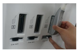
Figure 1-22. Lock the probe connection
