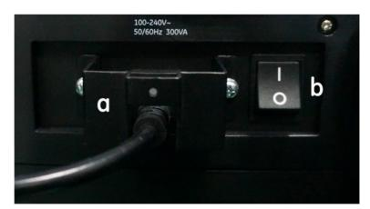
Figure 1-17. Circuit Breaker and Power Plug
