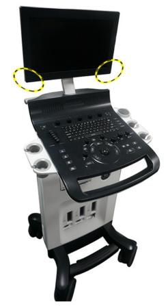
Figure 1-10. Grab the bottom of the monitor
