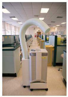
Fig. 1 The IQAir: FlexVac<sup>™</sup> air cleaning system used in this study
