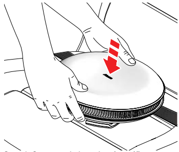
Step 4: Center and place the air purifier onto the car mount.
