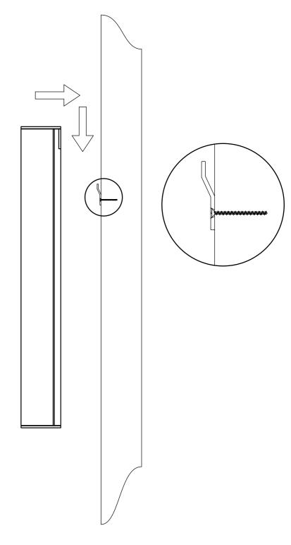
Step 3. Carefully take the mirror and lift on top of the wall bracket so that the rear panel of the mirror rests neatly up against the rubber pad of the bracket and make sure that it is roughly central on the bracket.
