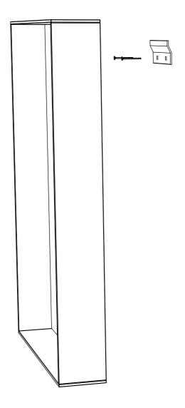
Step 1. Take the bracket and mark the holes for screws at the desired height, ensure that the bracket is straight using a spirit level.
