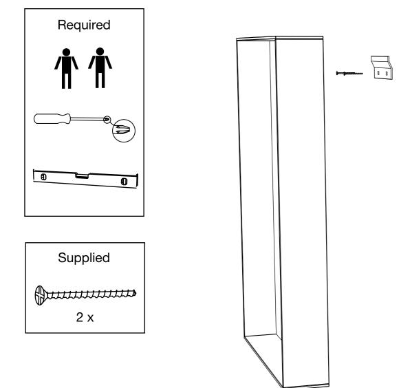
Step 1. Take the bracket and mark the holes for screws at the desired height, ensure that the bracket is straight using a spirit level.
