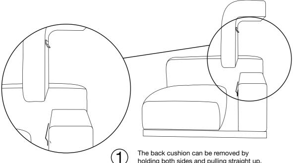
The back cushion can be removed by holding both sides and pulling straight up.
