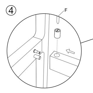
Insert fitting E into crossbar and add to the leg frame, fully tighten with screwdriver F.
