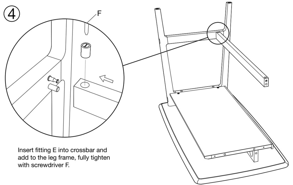
Insert fitting E into crossbar and add to the leg frame, fully tighten with screwdriver F.
