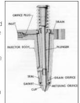
forced down and the preheated fuel charge is forced out through the six (seven in the NH) small holes of the injector cup into the cylinder (Fig. 10). These holes are only a few thousands of an inch in diameter and the fuel is completely broken up and distributed as a spray through the compressed air at the top of the cylinder.
