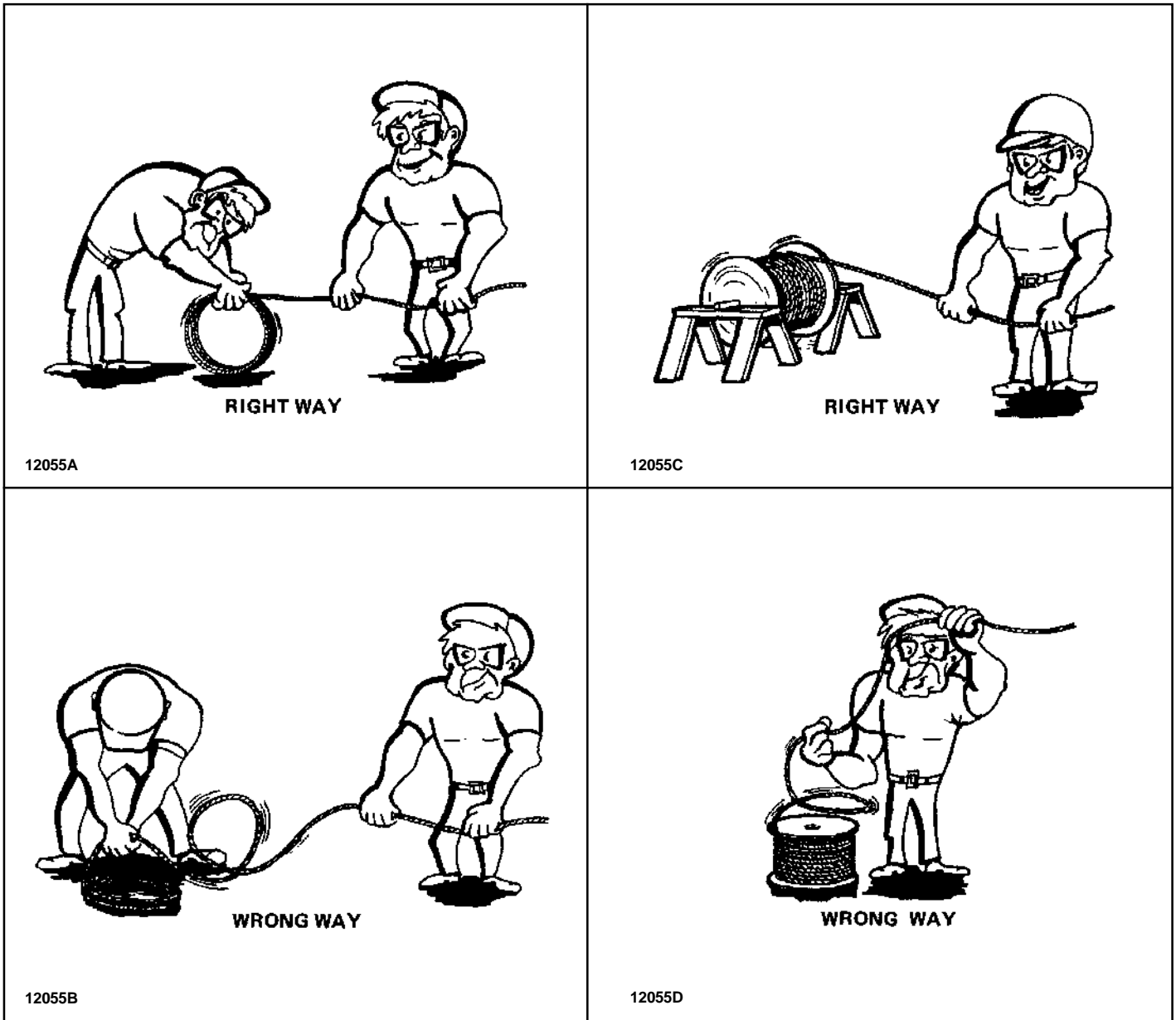
Figure 2-3. Rope Handling Instructions
