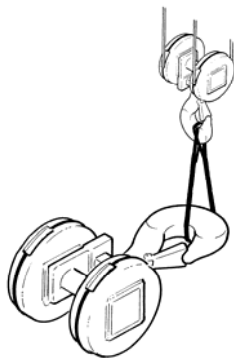
Figure 3-12 Lifting Bottom Block
