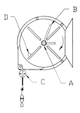
**INSTALLATION** - Mount the reel securely, Pull the grounding cable out to determine if the tension is sufficient for the intended use, If additional tension is needed, apply wrench to flats on the mainspring shaft (A), rotating counter-clockwise until the desired tension is reached.
