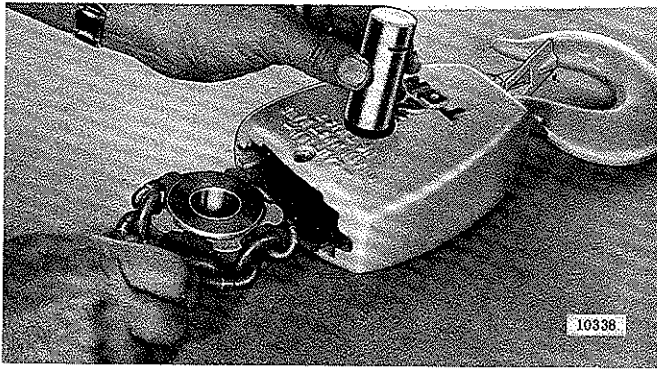
Figure 7-32. Removing Coil Chain and Sprocket on 2 and 3 Ton Lower Block Assembly (Coil Chain Model)
