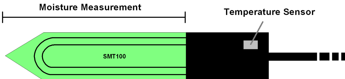
Figure 2: Sensor SMT100 with green capacitive measurement field and position of temperature sensor
