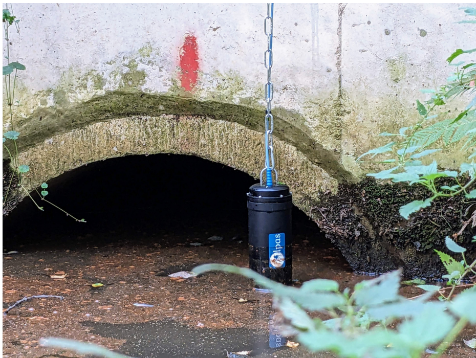
Figure 5. Olpas sensor (v1) installed in an overflow. Picture taken after overflow event.
