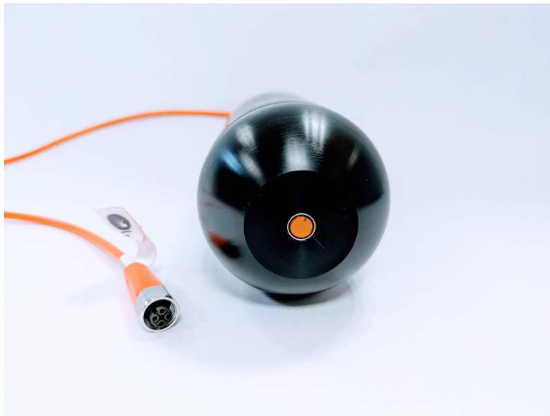
Figure 3. Full Olpas sensor seen from the top, with standard connector
