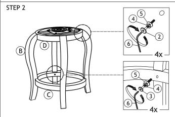
Attach part (B) with part (D). Tighten part (B) with part (D) first, then tighten part (B) with part (C) completely.
