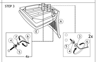
Insert 6 sets hardware first, then tighten part (A) with part (E) after alignment is done.
