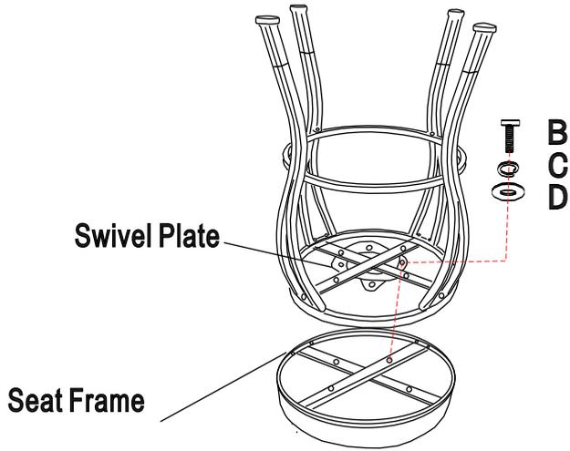
Attach swivel plate (G) to seat frame by using long allen bolt (B), spring washer (C) and flat washer (D) as shown
