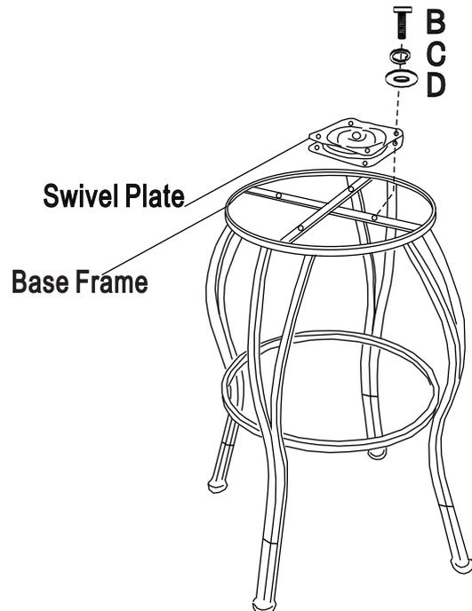
Attach swivel plate (G) to base frame by using long allen bolt (B), spring washer (C) and flat washer (D) as shown
