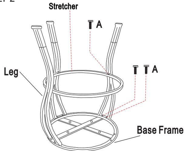
Attach three legs to base frame and stretcher by using short allen bolt (A) as shown
