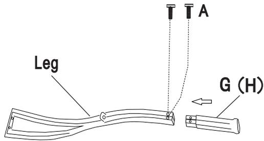
See Page 1 to determine the correct height you wish to assemble your stool. Insert four short feet (G) for counter height or long feet (H) for bar height in to the legs and secure by using short allen bolt (A) as shown
