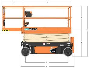
Platform Height - Elevated 7.8m A. Platform Height - Lowered 1.1m Platform Railing Height 1.1m Overall Height 2.2m Platform Dimensions 2.1 x 0.7m Platform Extension 0.86m Overall Machine Width 0.81m Overall Machine Length 2.4m Wheelbase 1.9m **Ground Clearance** 9.8cm
