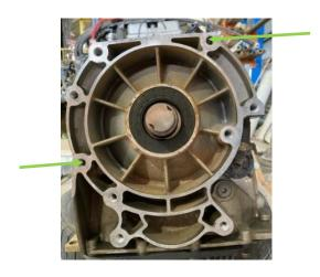
Please note - the torque specification for these 2 x special SHCS is 45 Nm = 33.19 Ft lbs.
