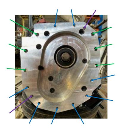
Please note - if you need to remove the SHCS in the future, the easiest way to do this is to apply a small amount of heat to the head of the SHCS using a small blow torch. Do not overheat the head or you may cause damage. If you are not confident in doing this, please have a qualified mechanic do it for you. Further, you must ensure that you do NOT use Loctite - Red Full Strength, as you will NEVER be able to remove the SHCS if the need arises.
