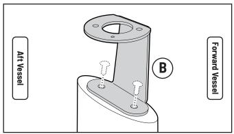
**Step 2**Connect cable to vessels lamp circuit. Use Supply Voltage between 10VDC and 30VDC (Typically 12 or 24 Volts systems).
