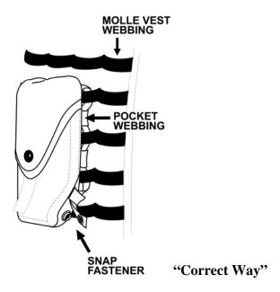
$\underline{\textbf{Do not}}$  simply place the attaching strap through the vest webbing without the interlocking weave. The pouches will not be secure if attached in this manner.
