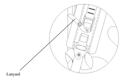
Emergency doffing can be accomplished by sharply pulling upward on the quick-release lanyard to disengage the buckle and letting the pack fall away.
