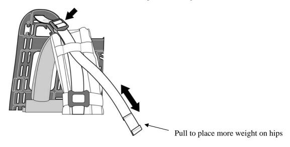
The ruck attachment straps are attached at the top slot on the frame with a three-bar buckle and webbing.
