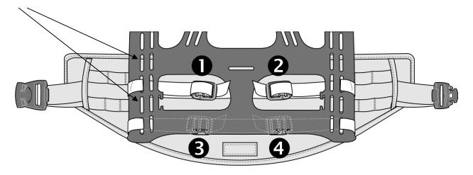
The load-lifter straps can be used to adjust the pack while marching. The weight of the pack can be transferred from the shoulders to the hips and back again by either cinching the 1" webbing down or by loosening the webbing by adjusting the non-slip buckle.
