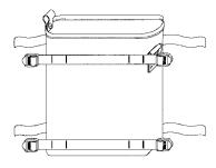
This removable pouch contains D-rings on each side to allow the radio to be carried by the General Purpose Sling when a pack is not needed. When the radio must be carried in the Large Ruck, the radio pouch is secured to the four black metal loops on the inside of the Large Ruck using the one-inch webbing.
