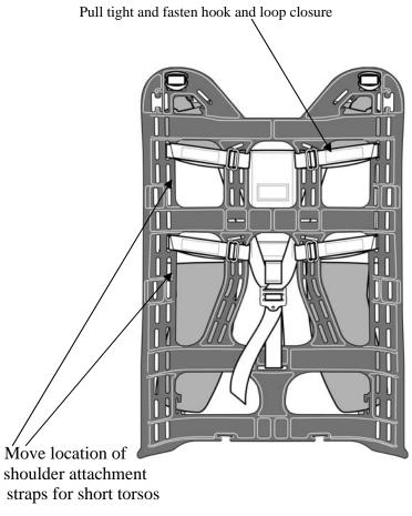
The waistbelt should be permanently connected to the frame utilizing 4 non-slip buckles as shown. For a short torso length, the waist belt can be moved as indicated in the illustration.
