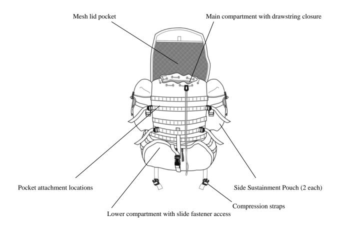
The MOLLE Large Ruck capacity is 4000 cubic inches. The side sustainment pouch capacity is 500 cubic inches each.
