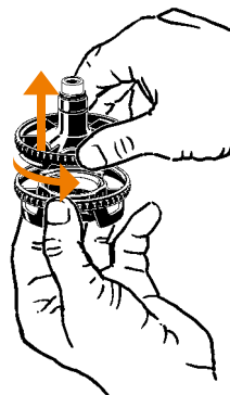
Remove Filling Chamber Cap
