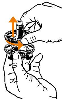
Remove Filling Chamber Cap
