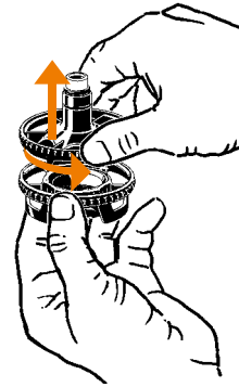
Remove Filling Chamber Cap
