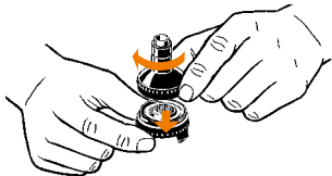
Screw on Filling Chamber Cap
