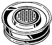
The Dosing Capsule inserted into the Dosing Capsule Adapter
