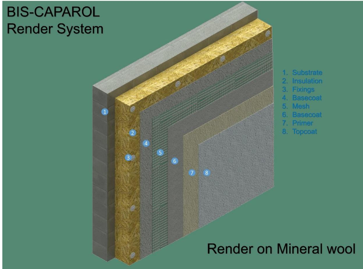
A1 Non combustible BRE fire accredited mineral wool Insulation is fixed to the solid substrate using the insulation fixings. Insulation fixings are as per the standard fixings minimum of 5 fixings per board. A layer of basecoat is applied on top of Insulation. Reinforced mesh is then attached to the applied base coat. A 2nd layer of base coat is applied on top of the reinforced mesh, and then patches and additional reinforced mesh is applied on the openings.
